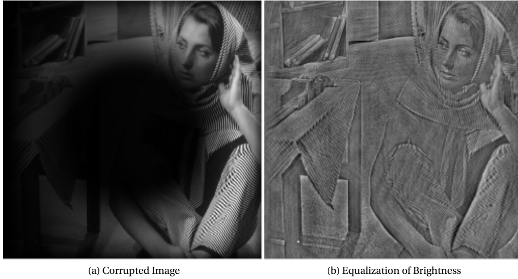
Figure 5.8: (a) Artificially corrupted image. Gray levels are multiplied by a ramp function and by 0.05 in the center. (b) Reconstruction from phase only. The brightness is now balanced, in particular the difference of brightness between the dark center and its outside disappears. Even fine image structures are recovered. Decomposition was computed using k = 5 sub-channels.
