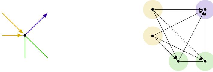
**Figure 3.1:** The construction of a line graph for mixed graphs. Every arc or edge in the original graph (left) is associated with a vertex in the line graph (right). Vertices representing two incident edges are connected by an edge. Vertices representing two incident arcs/edges which form a path are connected by an arc.
