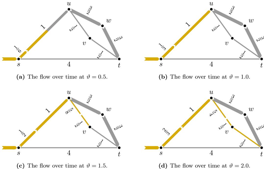
Figure 4.3: A flow over time along the path  $s-u-v-t$  through the network depicted in Figure 4.2. Every arc  $a$  is annotated with its respective queuing delay  $q_a(\vartheta)$  (if it is nonzero) and its transit time  $\tau_a$ . The relative contributions of  $q_a(\vartheta)$  and  $\tau_a$  to the total transit time  $q_a(\vartheta) + \tau_a$  is indicated by a small gap in the link.
