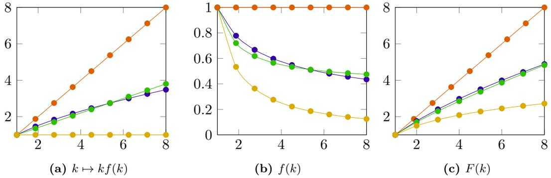
**Figure 5.1:** The relevant cost functions under constant total edge cost (yellow), polynomial total edge cost with  $\alpha = 0.6$  (violet), affine total edge cost with  $s = 0.4$  (green), and linear total edge cost (red).
